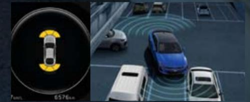
**Parking Distance Warning (PDW)** For utmost confidence and peace of mind when maneuvering into and out of tight parking spaces, PDW uses ultrasonic sensors mounted on the front and rear bumpers to warn you of any nearby obstacles.
