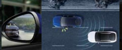
**Blind-Spot Collision Warning (BCW)** At speeds of 20 km/h or higher, BCW alerts you if a vehicle enters your blind spot, even when you are in the process of changing lanes. LED warnings flash on the door mirror and an audio warning is emitted when you signal to make a lane change.
