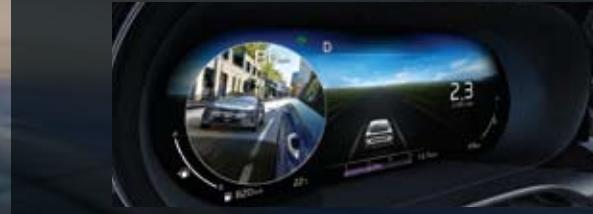
**Blind-Spot View Monitor (BVM)** Signal a lane change and, if there is a possibility of a collision, BVM will show live video footage on the instrument cluster of what's in the blind spots of the outside mirror on the side of your intended lane change.
