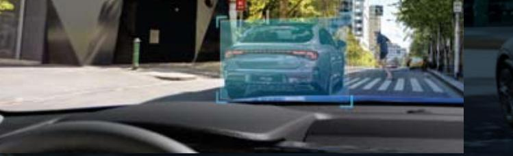
**Forward Collision-Avoidance Assist (FCA)** FCA uses a front-view camera and front radar to detect vehicles, pedestrians or cyclists ahead. By warning the driver and automatically applying the brakes, FCA helps to avoid or reduce the severity of an accident.
