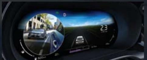
**Blind-Spot View Monitor (BVM)** Signal a lane change and, if there is a possibility of a collision, BVM will show live video footage on the instrument cluster of what's in the blind spots of the outside mirror on the side of your intended lane change.
