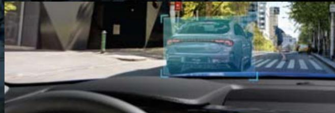
**Forward Collision-Avoidance Assist (FCA)** FCA uses a front-view camera and front radar to detect vehicles, pedestrians or cyclists ahead. By warning the driver and automatically applying the brakes, FCA helps to avoid or reduce the severity of an accident.
