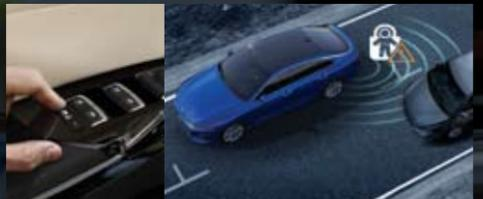
**Safe Exit Assist (SEA)** Using the K5's rear corner radar, SEA detects cars approaching from behind and cautions passengers who may intend to exit the vehicle. SEA will even override Electronic Child Safety Lock settings until the approaching vehicle has passed.
