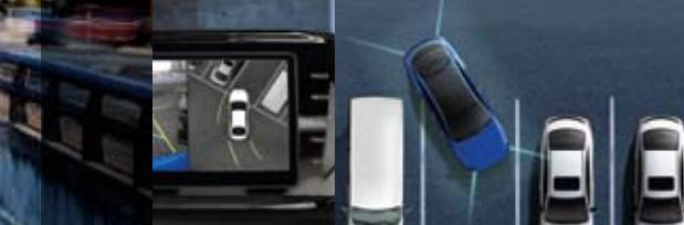
**Surround View Monitor (SVM)** When operating in confined spaces, multiple cameras provide you with a zoomable, 360° overhead view of the vehicle's surroundings, so you can maneuver with confidence and without having to get out of the vehicle.
