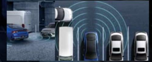
**Rear Cross-Traffic Collision Warning (RCCW)** The RCCW radars detect the presence of cross traffic in the lane the K5 is backing into. If a vehicle is detected on either side, an audible warning will sound, and a cluster warning graphic will illuminate, until the path is clear.
