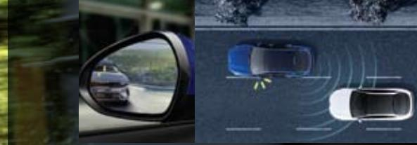
**Blind-Spot Collision Warning (BCW)** At speeds of 20 km/h or higher, BCW alerts you if a vehicle enters your blind spot, even when you are in the process of changing lanes. LED warnings flash on the door mirror and an audio warning is emitted when you signal to make a lane change.
