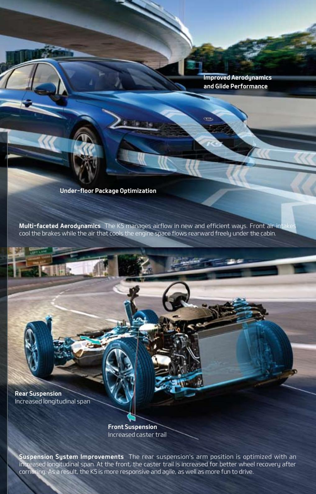
**Suspension System Improvements** The rear suspension's arm position is optimized with an increased longitudinal span. At the front, the caster trail is increased for better wheel recovery after cornering. As a result, the K5 is more responsive and agile, as well as more fun to drive.
