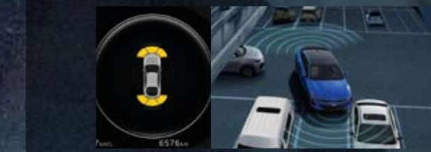
**Parking Distance Warning (PDW)** For utmost confidence and peace of mind when maneuvering into and out of tight parking spaces, PDW uses ultrasonic sensors mounted on the front and rear bumpers to warn you of any nearby obstacles.
