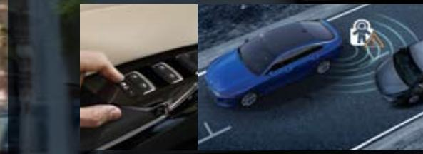
**Safe Exit Assist (SEA)** Using the K5's rear corner radar, SEA detects cars approaching from behind and cautions passengers who may intend to exit the vehicle. SEA will even override Electronic Child Safety Lock settings until the approaching vehicle has passed.
