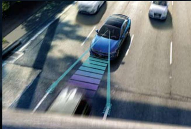
**Smart Cruise Control (SCC)** SCC maintains the driver's selected speed and, using the front-view camera and front radar, helps to maintain a safe following distance. SCC will reduce speed and even stop the car when needed. Then when the car ahead moves, SCC automatically accelerates for you. SCC is now activated with the simple touch of a button.
