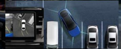
**Surround View Monitor (SVM)** When operating in confined spaces, multiple cameras provide you with a zoomable, 360° overhead view of the vehicle's surroundings, so you can maneuver with confidence and without having to get out of the vehicle.
