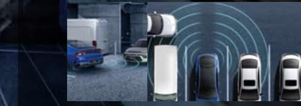
**Rear Cross-Traffic Collision Warning (RCCW)** The RCCW radars detect the presence of cross traffic in the lane the K5 is backing into. If a vehicle is detected on either side, an audible warning will sound, and a cluster warning graphic will illuminate, until the path is clear.
