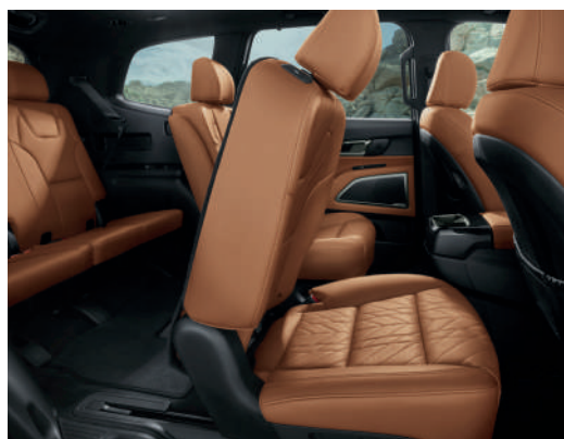
One-touch slide and fold 2nd-row seats slide and fold forward to give 3rd-row passengers easy access.
