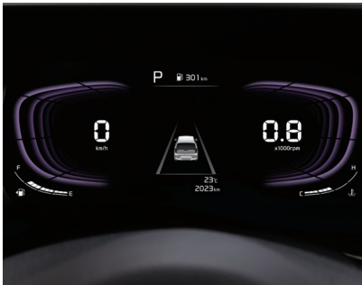
Supervision cluster (4.2-inch color TFT LCD)
