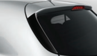
Rear spoiler garnish A rear spoiler improves the air vortex around C-pillar for enhanced aerodynamics and downforce on the rear tires.
