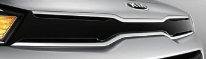
Radiator grille The iconic Kia radiator grille has been completely restyled. Most of the airflow used for cooling enters through the lower intake.
