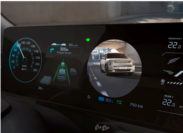
Blind-Spot View Monitor (BVM) displays the rear-side image of the corresponding direction when the turn signal switch is engaged.
